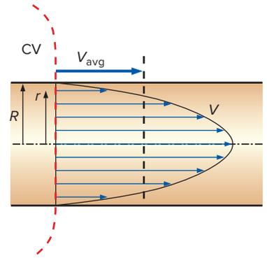
**FIGURE 13–22** Velocity profile over a cross section of a pipe in which the flow is fully developed and laminar.
