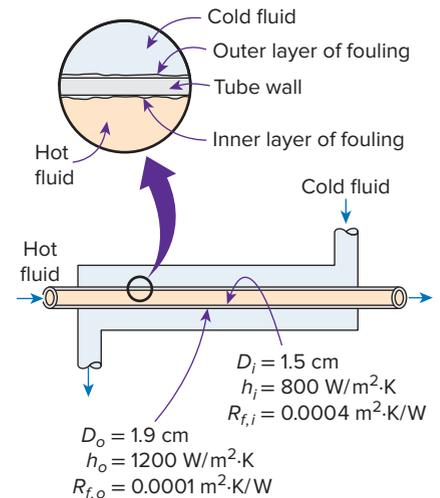
FIGURE 22–12 Schematic for Example 22–2.
