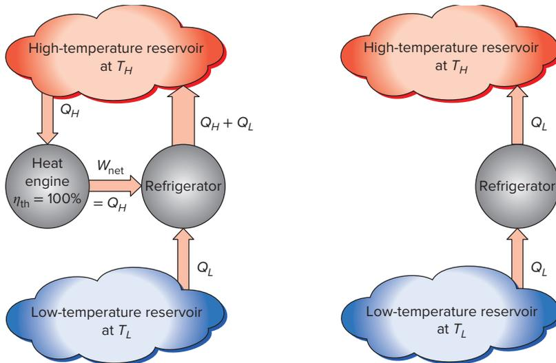
(a) A refrigerator that is powered by a 100 percent efficient heat engine
