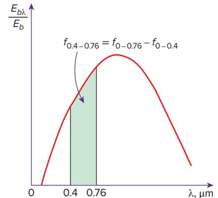
**FIGURE 21-15** Graphical representation of the fraction of radiation emitted in the visible range in Example 21-2.
