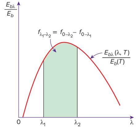
**FIGURE 21-14** Graphical representation of the fraction of radiation emitted in the wavelength band from  $\lambda_1$  to  $\lambda_2$ .
