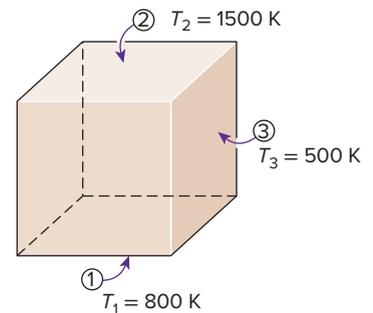
**FIGURE 21-47** The cubical furnace of black surfaces considered in Example 21-9.
