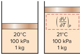
(a) A substance with a large  $\beta$
