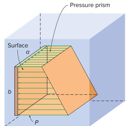
**FIGURE 11-7** The hydrostatic forces acting on a plane surface form a pressure prism whose base (left face) is the surface and whose length is the pressure.
