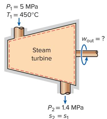
**FIGURE 8-15** Schematic and  $T$ - $s$  diagram for Example 8-5.
