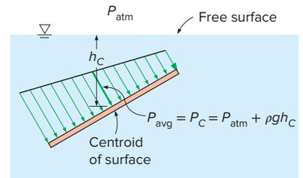
**FIGURE 11-4** The pressure at the centroid of a plane surface is equivalent to the *average* pressure on the surface.
