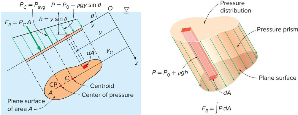
**FIGURE 11-3** Hydrostatic force on an inclined plane surface completely submerged in a liquid.
