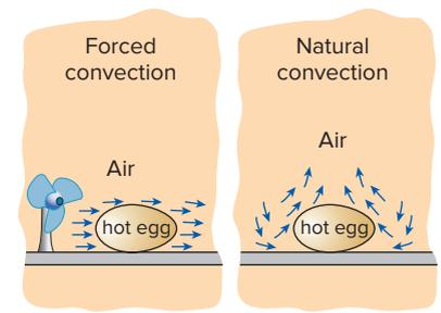
**FIGURE 16–12** The cooling of a boiled egg by forced and natural convection.
