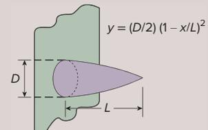
**Pin fins of parabolic profile (blunt tip)**
