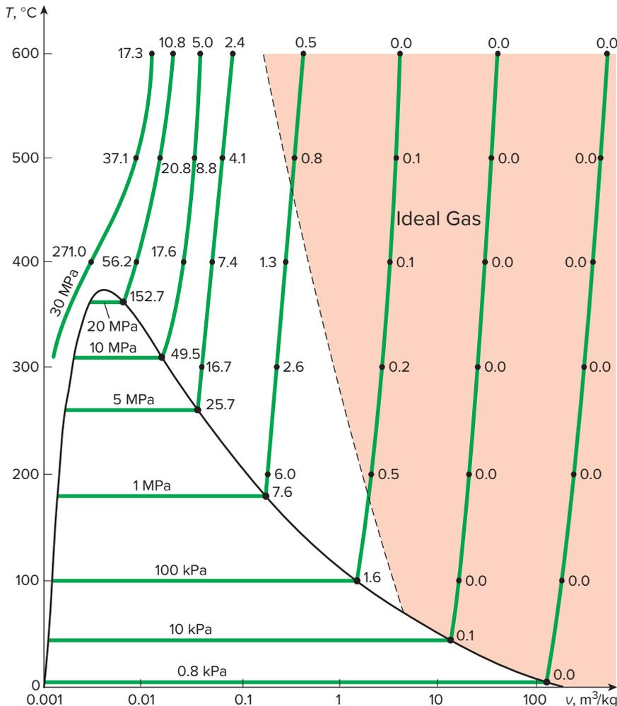
**FIGURE 4–45** Percentage of error involved in assuming steam to be an ideal gas, and the region where steam can be treated as an ideal gas with less than 1 percent error.
