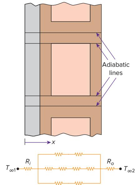
**FIGURE 17–22** Alternative thermal resistance network for Example 17–6 for the case of surfaces parallel to the primary direction of heat transfer being adiabatic.
